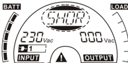
■ Figure 6.5 The Fault mode
