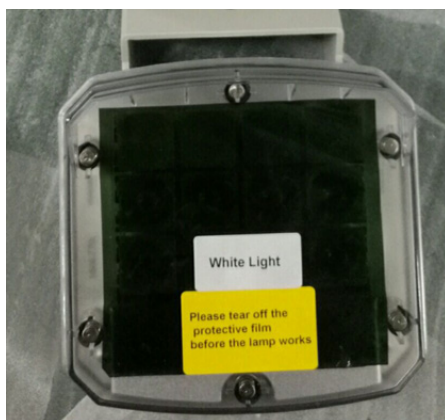
Figure 2. Protective Film Covering an White Illuminator (left), Protective Film Covering an IR Illuminator (right)
