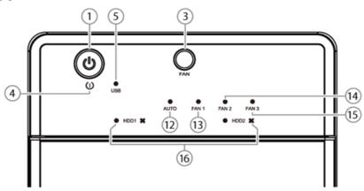
1. Power Button It needs to be PRESSED AND HELD for 3 seconds to power off.
