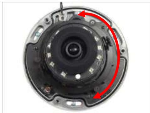
3. To tilt the lens, loosen the two (2) tilt adjustment screws. Then, adjust the tilt and tighten back the screws to fix the tilt position.
