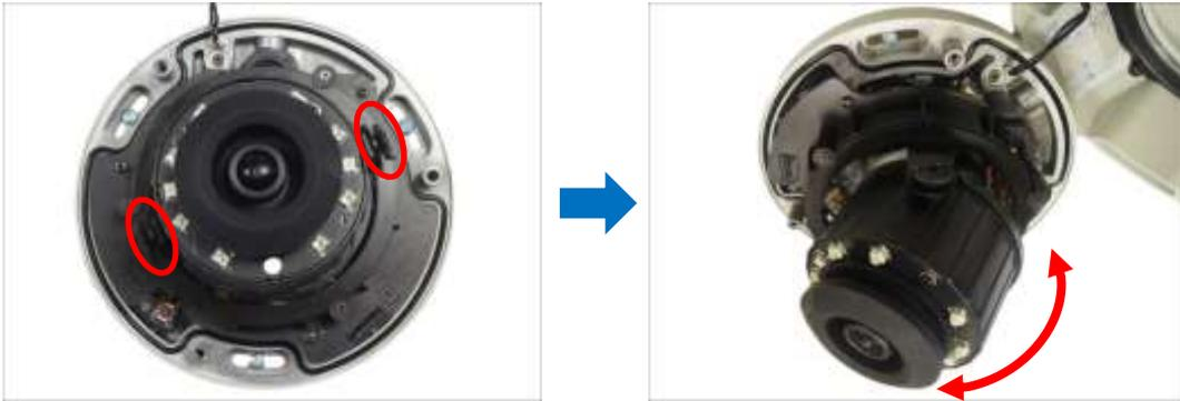
4. To rotate the video orientation, turn the lens module left or right.
