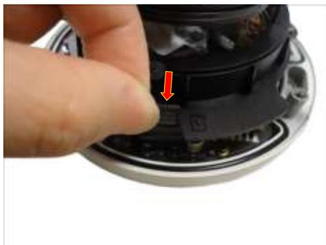
3. Push the card completely into the slot.
