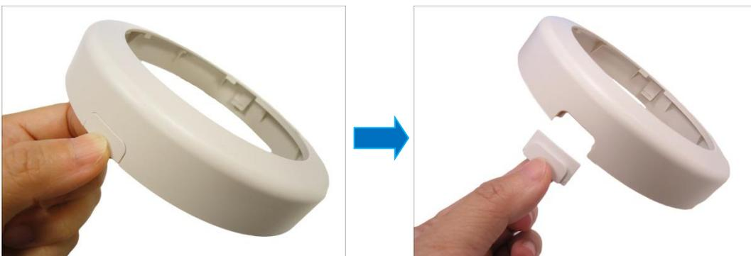
3. Install a memory card into the memory card slot of the camera, as needed.
