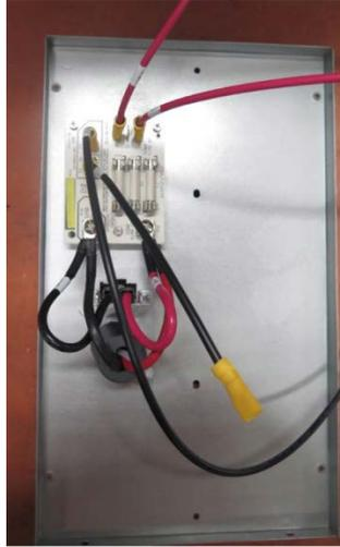
2. Please assemble the 12PCS batteries with black wire into the Battery Case as below.
