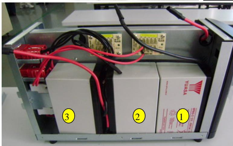
7. Put the three batteries in order as shown in chart. **Hint:** Install the left one and keep battery terminal heading the bottom. Then, install the middle one and keep battery terminal heading upwards. At least, install the right one and keep battery terminal heading upwards.
