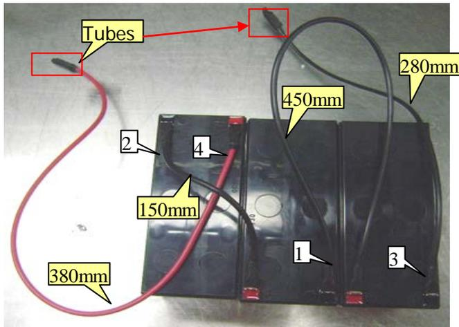
5. As shown, please use three batteries (12V/7Ah or 12V/9Ah) and check the date code (it's necessary to use batteries with same date code in a UPS unit). Serial connect batteries with three black wires in 450, 280, 150 mm length. Slip the end of black wire with 280mm length into the tube.
