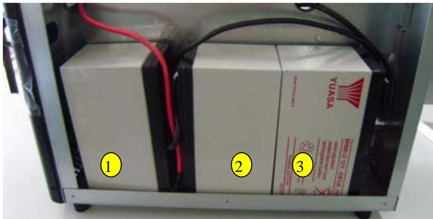
3. Put the three batteries in order as shown in chart. **Hint: Install the left one and keep battery terminal heading the bottom. Then, install the middle one and keep battery terminal heading upwards. At least, install the right one and keep battery terminal heading upwards.**
