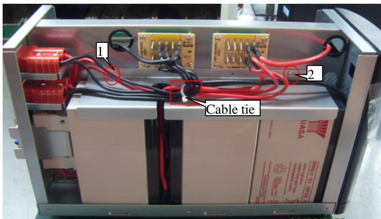
8. Put grommet inside the hole of battery divider and allow red and black wire passing through the hole. Screw tightly the battery divider with screw nuts. (as shown in 1, 2 areas)
