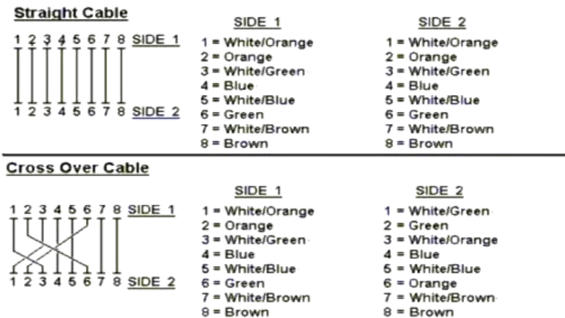
Figure A-1: Straight-Through and Crossover Cable
