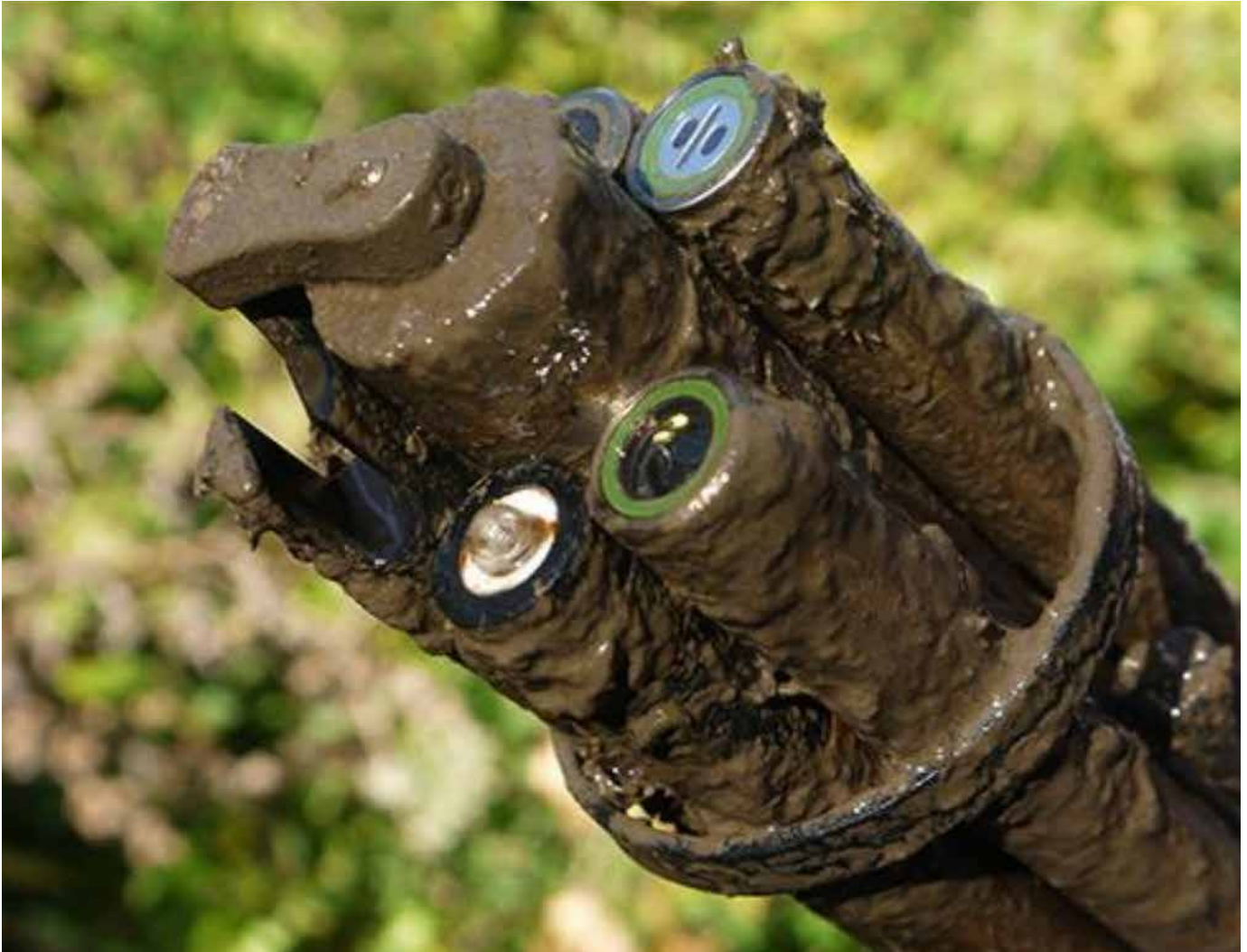
Figure: Typical fouling on the Eureka Manta sensor probes
