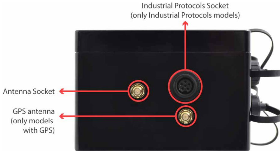
Figure: Antenna side of the enclosure
