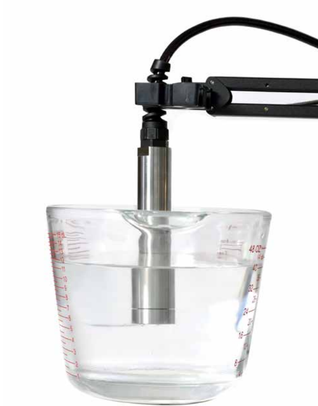
Figure: Immersing the sensor inside the calibration buffer solution
