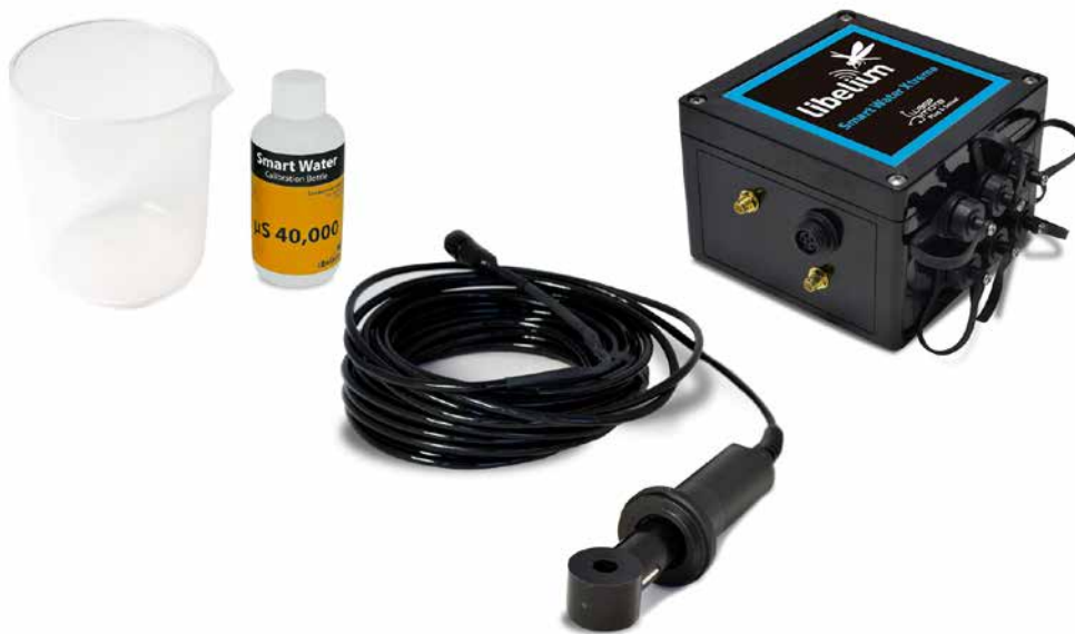
Figure: Necessary elements for CTZN sensor probe calibration
