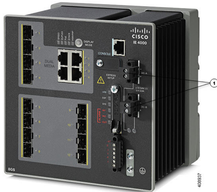
Figure 10 Removing the Power Connectors from the Switch
