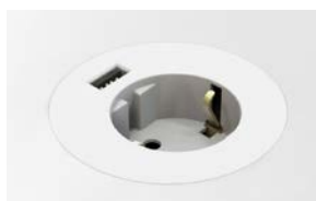
935-PM61W POWERDOT MIDI, WHITE 1 POWER, 1 USB-CHARGER (2.1A) 1.55 M CONNECTION (SCHUKO) FIXED LEVEL, HEIGHT 82.1 MM
