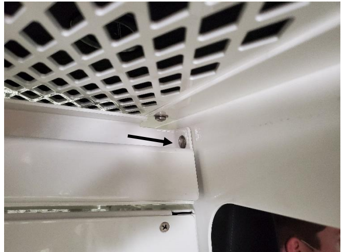
Attach to upper front bulkhead using 1/4" x 3/4" carriage bolts and serrated nuts.
