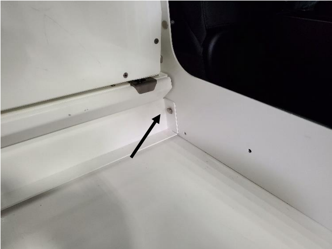
Attach divider to lower front bulkhead using 1/4" x 3/4" carriage bolts and serrated nuts.
