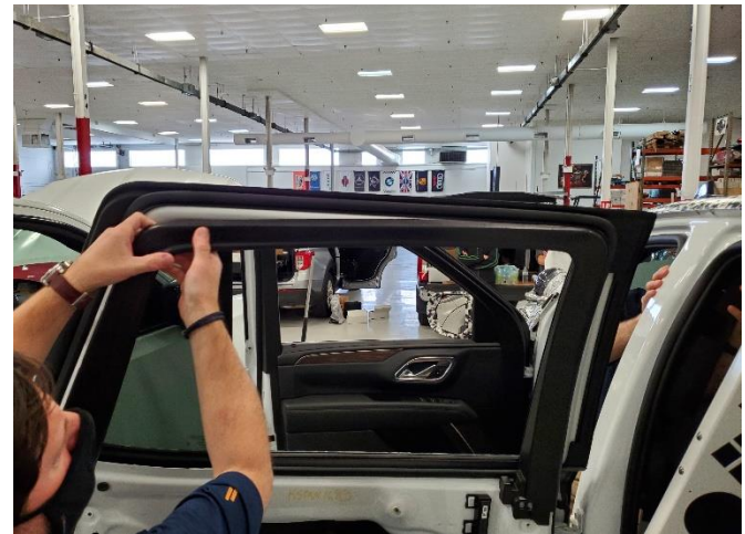
Gently remove trim around window frame.
