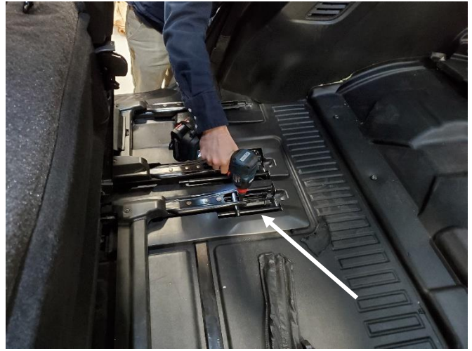
Flip seat seats forward to access hardware.
