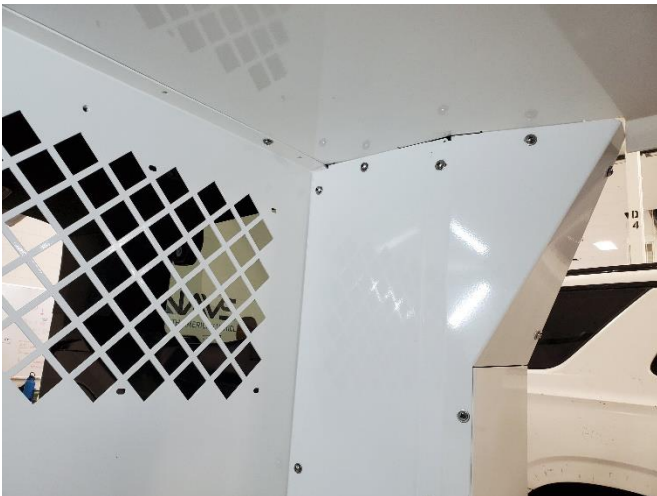
Attach trim to rear wall and ceiling with 1/4" x 3/4" Phillips head bolts and flat washers.
