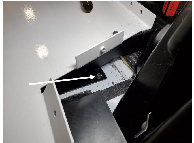
Tighten rear floor mounting hardware.
