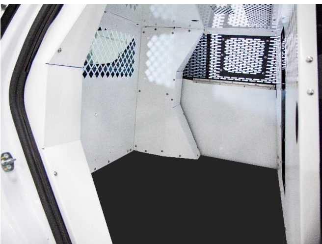
Place rubber mat into kit after silicone is dry.
