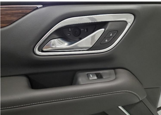
Remove plastic covers behind the paddle handle. Remove screws. (7mm socket)
