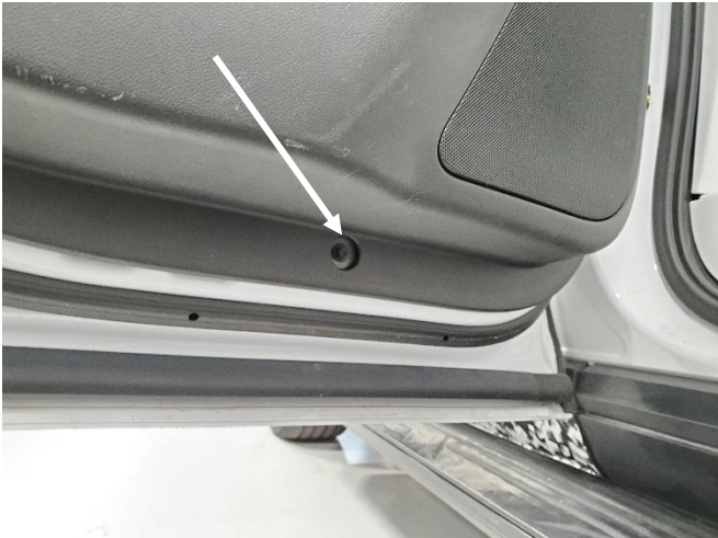
Remove screw at bottom of door panel. (7mm socket)
