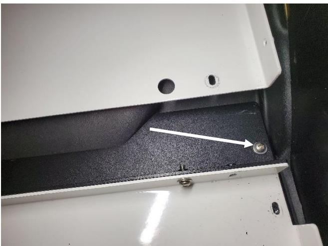
Cargo filler will also attach to floor mounting brackets in corners with 1/4" x 3/4" Phillips head bolts and flat washers.
