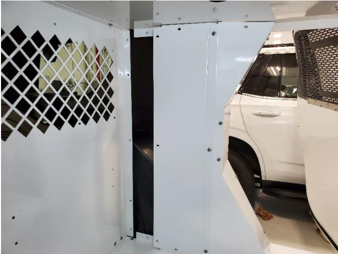
Place side filler assembly into kit and slide towards rear bulkhead.
