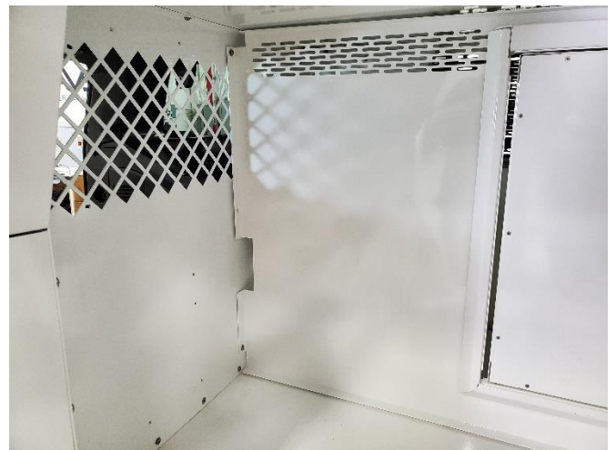
If installing optional K9-A-115 divider, place into insert and line up to threaded inserts in the rear of the kit. Attach using 1/4" x 3/4" Phillips head bolts and flat washers.
