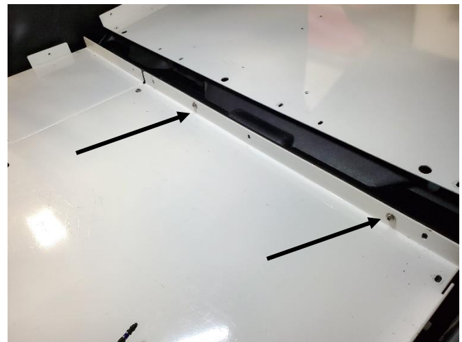
Attach rear cargo, filler plate to floor using 1/4" x 3/4" Phillips head bolts and flat washers.
