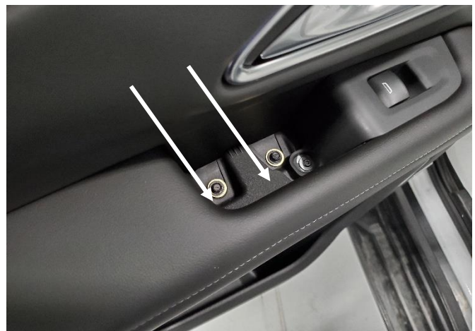
Remove plastic covers behind armrest handle. Remove screws. (7mm socket)
