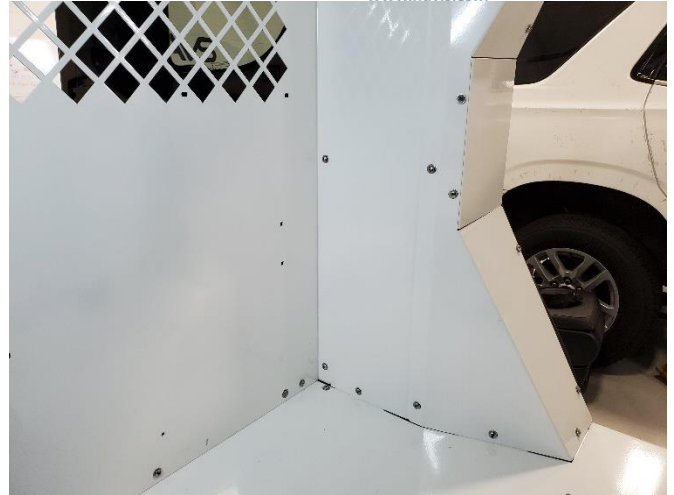
Square up kit and loosely attach side trim to floor with 1/4" x 3/4" Phillips head bolts and flat washers.
