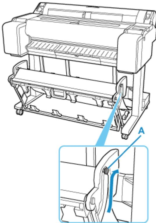
2. When using 24-inch or A1 (portrait) roll paper, pull out the Adjustable Stopper (B).
