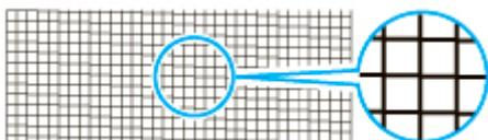
If some sections of the horizontal lines are faint or incomplete, the nozzles for those colors are clogged.
