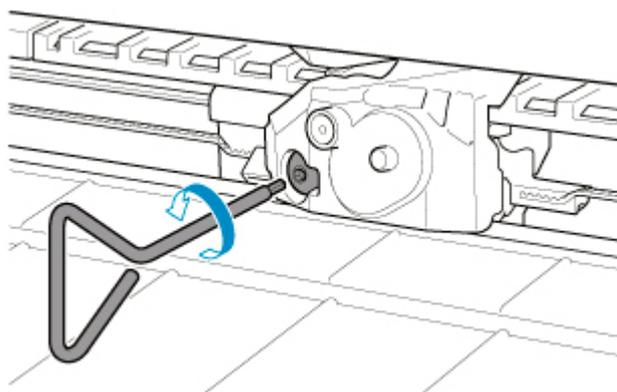
7. Remove cutter blade while holding A.
