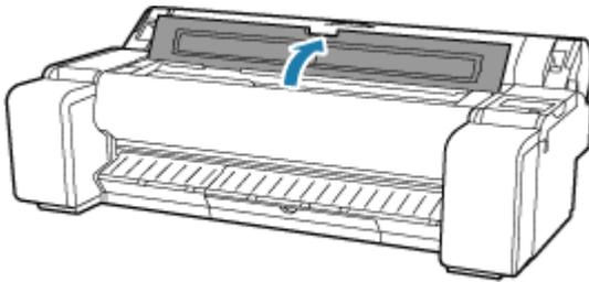
6. If the print head locking cover and print head lock lever are dirty, use a damp cloth that you have wrung out completely to wipe them clean.
