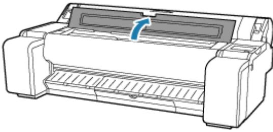
7. Align the angle adjustment lever with the red square and close the top cover.
