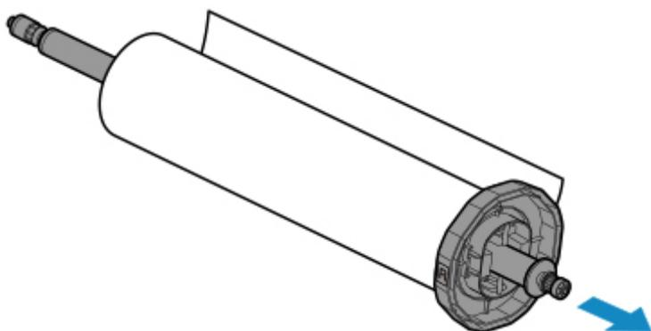
3. To remove 3-inch paper core attachment, press tabs (A) inward and remove attachment.
