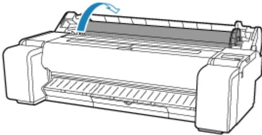
7. Hold roll holder by its flanges (A) and remove from roll holder slot.
