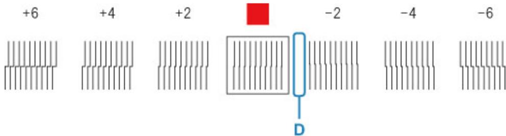
9. Open top cover and move angle adjustment lever to match number (or square) of straightest set of lines.
